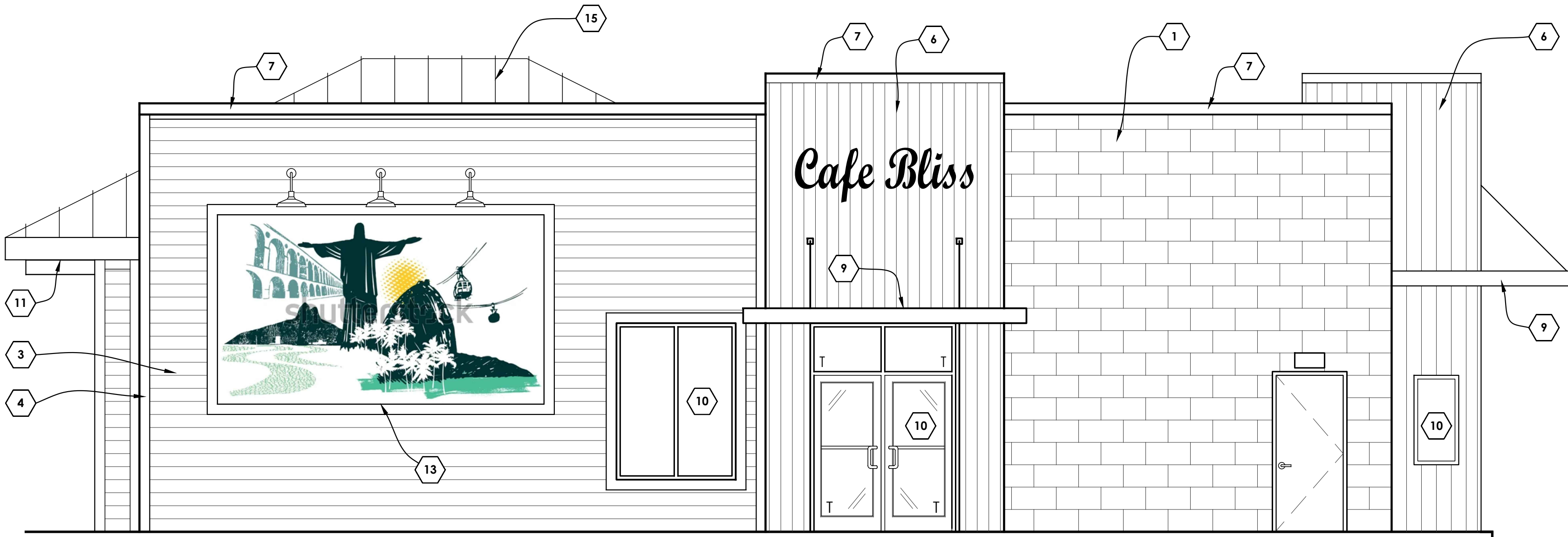
2 EAST SIDE (ENTRY / PARKING) ELEVATION A-201 SCALE: 1/4" = 1'-0"
