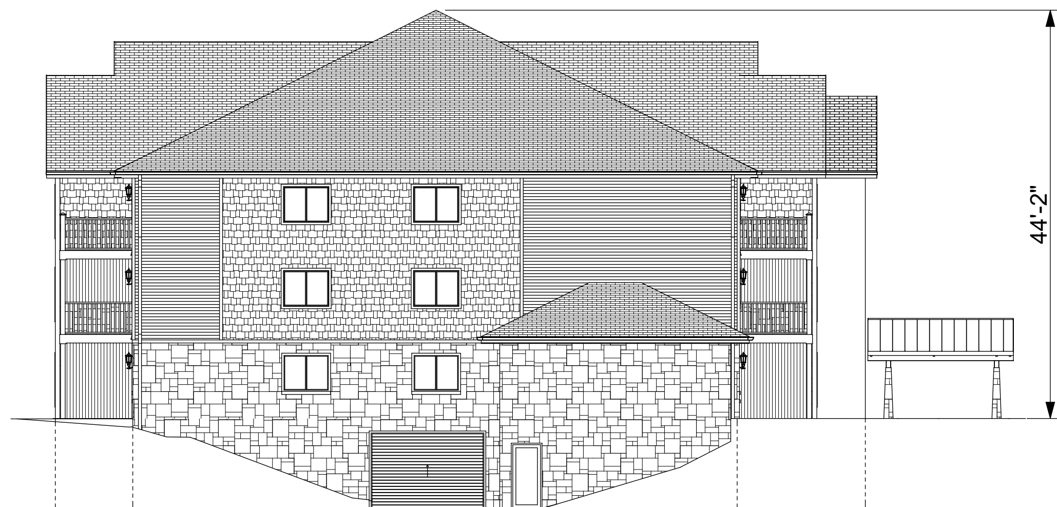
Side Elevation at Garage Entry
