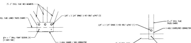
DETAIL 6-HOLE WEB CONNECTOR NOT TO SCALE
