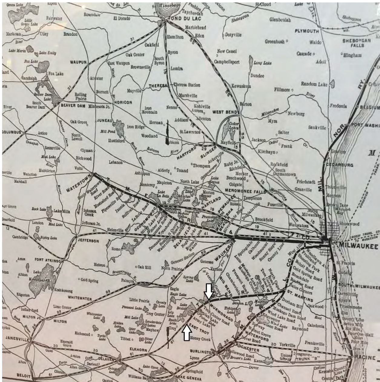
Historic Map 04 of The Milwaukee Electric Railway & Light Company's network of electric railroads and connecting bus lines, c. 1930. Arrows show the current section of the East Troy Electric Railroad with termination points in East Troy and Mukwonago. The bolder dashed lines are rail lines while the lighter dashed lines are bus routes, such as the one leaving East Troy to the west.
